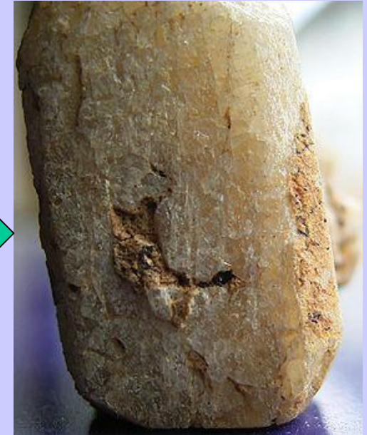
Anorthite (plagioclase calcique) \text{CaAl}_2\text{Si}_2\text{O}_8 T^\circ \text{ fusion} = 1550^\circ \text{C}
