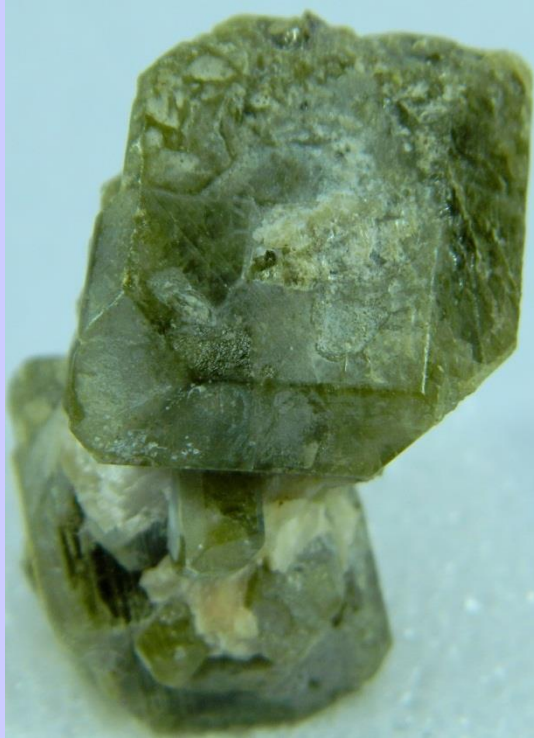
Diopside (clinopyroxène) \text{CaMg}(\text{Si}_2\text{O}_6) T^\circ \text{ fusion} = 1391^\circ \text{C}
