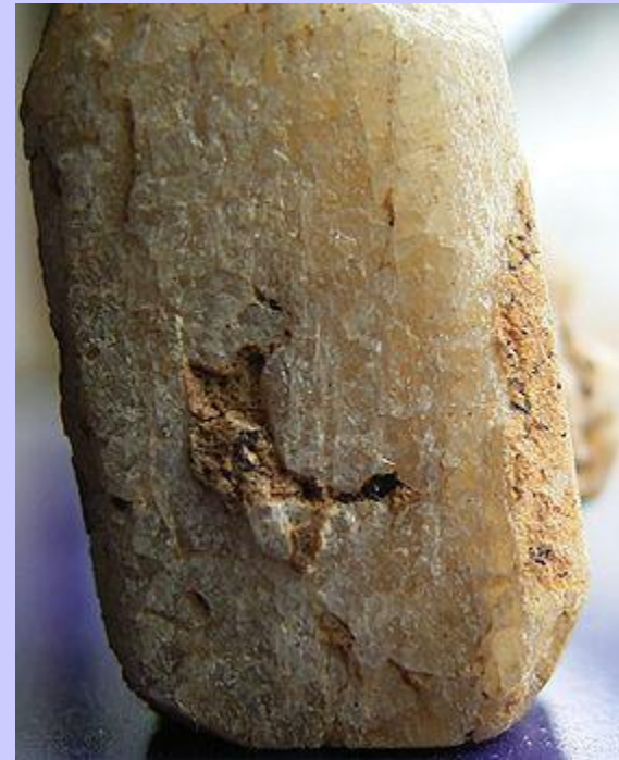
Anorthite (plagioclase) \text{CaAl}_2\text{Si}_2\text{O}_8 T^\circ \text{ fusion} = 1550^\circ \text{C}
